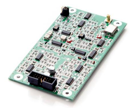
SEXC23COD2 board is a full multiplex stereo encoder specially designed to be incorporated in Sielco transmitters. It incorporates the left and right 15kHz channel filters and the management of the monophonic transmission, but not the pre-emphasis network which is managed by the transmitter. The card is easily installed in the factory or on the field on any Sielco FM or STL Transmitter of the EXCxxGT/GX, EXC18 and EXC19 series.
